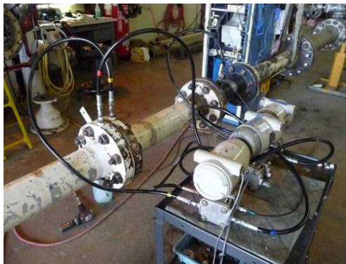
Fig 5. CEESI 4" orifice meter test set up.
