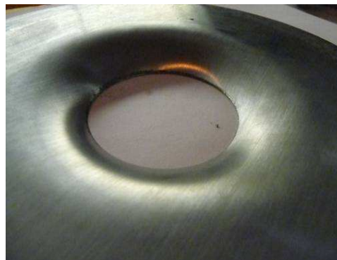
Fig 6. Buckled Plate (sharp edge upstream).
