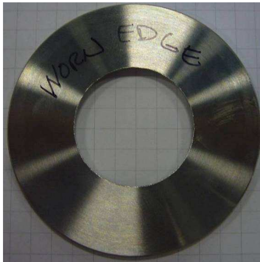
Fig 11. Worn Orifice Edge.
