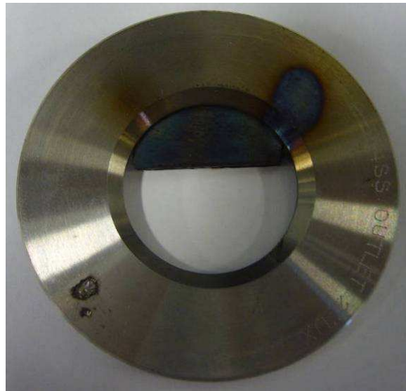
Fig 8. An Partially Blocked Orifice Plate.
