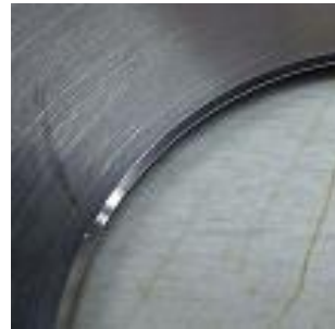
Fig 20. Chamfered (0.02”) orifice edge.
