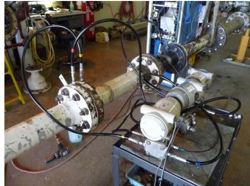
Fig 5. Flange installed plate with air flow.
