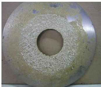
Fig 23. A heavily contaminated orifice plate.
