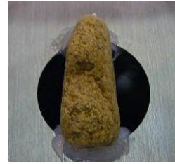
Fig 30. Rock trapped at an orifice plate.
