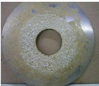
Fig 14. Contaminated Orifice Plate.
