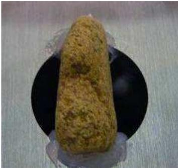
Fig 16. Rock Trapped at an Orifice Plate.
