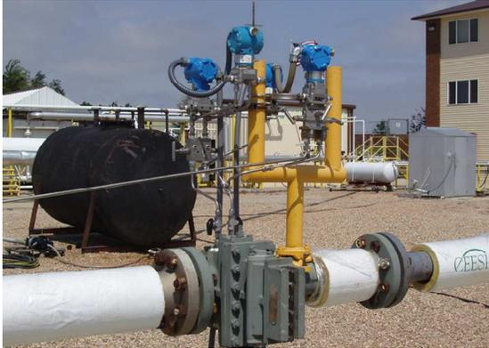
Fig 21. Wet gas flow test of an orifice meter with pressure taps at top dead centre.
