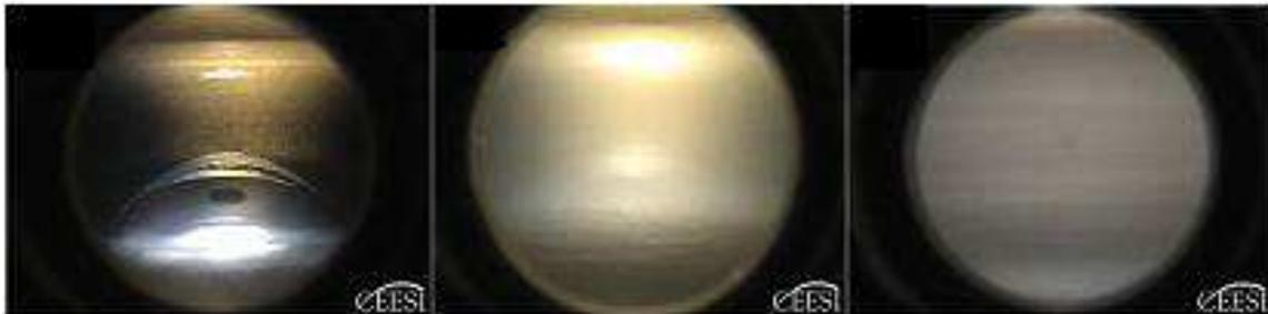
Fig 23a. Gas/HCL stratified. Fig 23b. Gas/HCL transition. Fig 23c. Gas/HCL annular.
