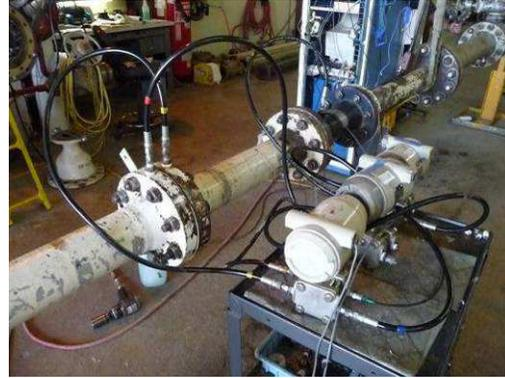
Fig 4. Flange installed plate with air flow.
