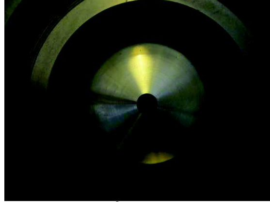
Fig 23. Approx 1° misaligned cone.
