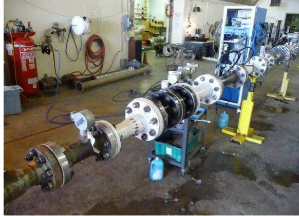
Fig 12. 3" Swirl Generator + Expansion 9D up
