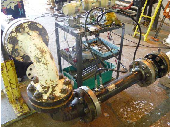
Fig 7. DOPB 0D up & HMOP 2D down
