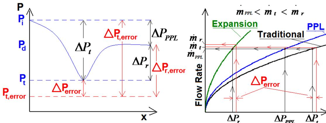
Fig 30. Graphical representation on the effect of an artificially low throat pressure.
