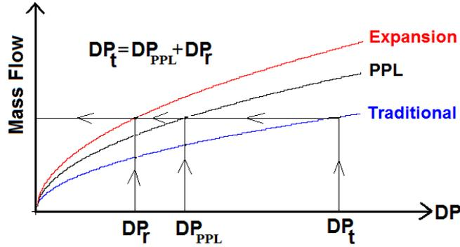
Fig 29. Sketch (not to scale) showing typical DP's and flow equations relationships.
