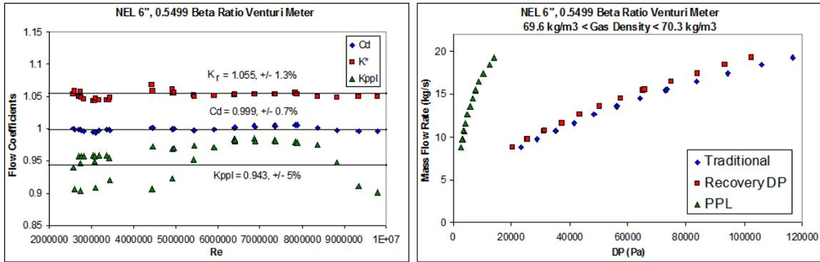
Fig 25. ISA Controls 6", sch 80, 0.55 Beta Ratio Venturi Meter with Short Downstream Pressure Tapping.
