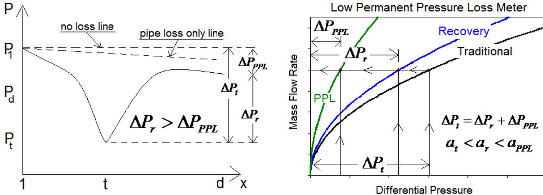
Fig 5a. Pressure fluctuation through DP meter where majority of DP is recovered (PLR < 1/2) and the associated three parabolic flow rate equations.
