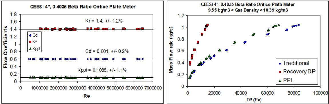
Fig 8. CEESI Wet Gas JIP 4", 0.4035 Beta Ratio Orifice Plate Meter Dry Gas Data.
