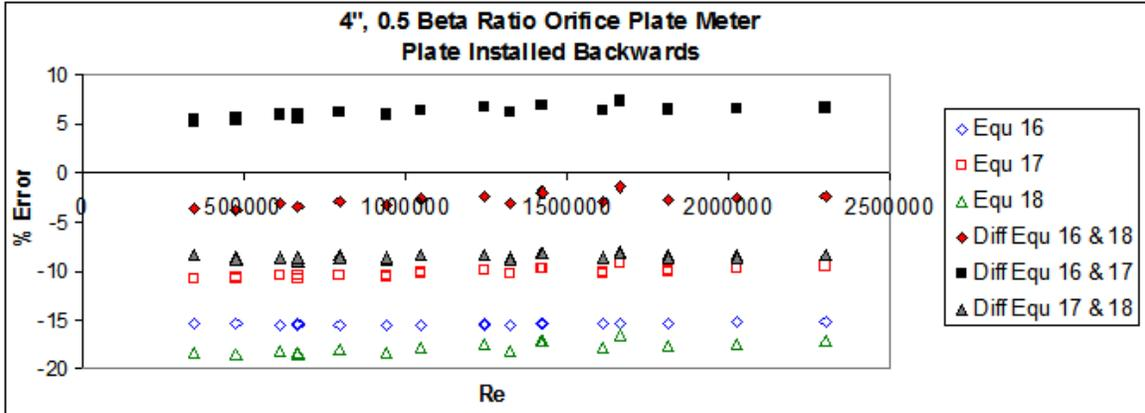
Fig 34. CEESI 4", Sch 40, 0.5 Beta Ratio Orifice Plate Meter with Plate Installed Backwards.
