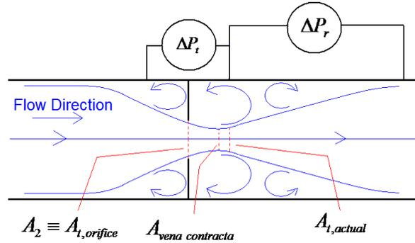
Fig A1. Sketch of Typical Flow Through an Orifice Plate Flow Meter.
