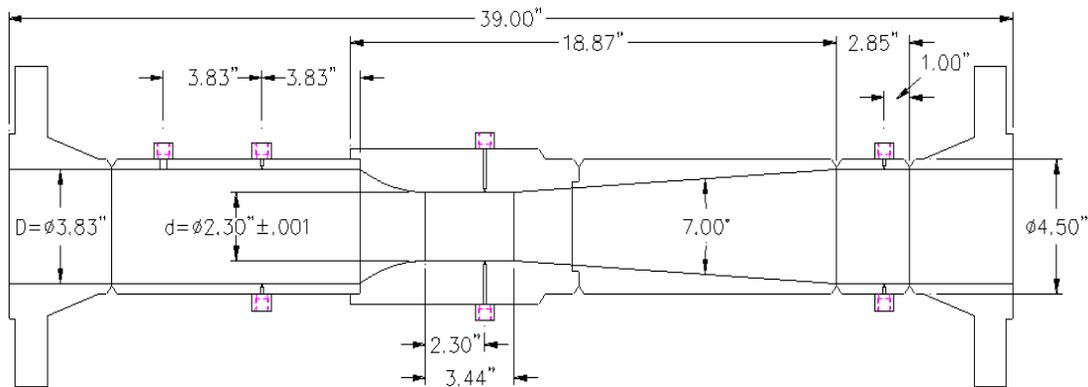
Fig 26. CEESI 4", 0.6 Beta Ratio Circular Arc Inlet Venturi Meter.
