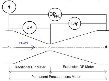
Fig 4. Venturi Meter with 3 DP measurements.
