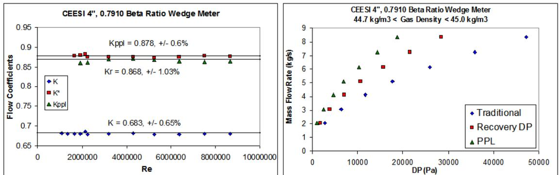
Fig 20. CEESI Wet Gas Facilities Commissioning 4", 0.7910 Beta Ratio Wedge DP Meter Dry Gas Data.
