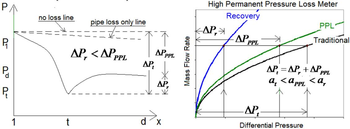
Fig 5b. Pressure fluctuation through DP meter where majority of DP is lost (PLR > 1/2) and the associated three parabolic flow rate equations.
