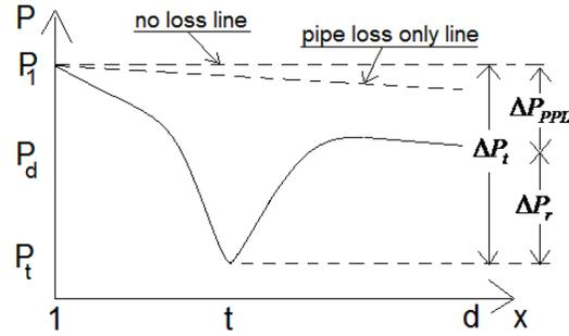
Fig 4a. Sketch of DP Meter Pressure Fluctuations.
