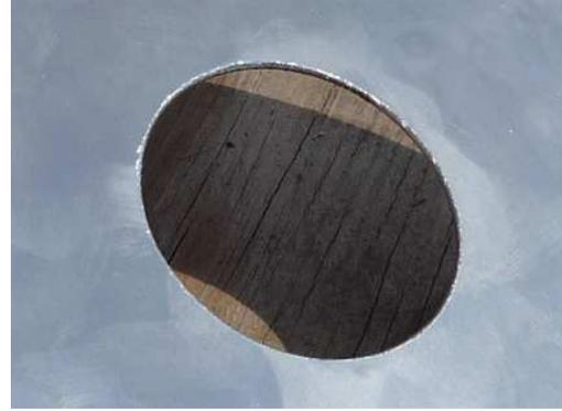
Fig 33b. Sharpness of Orifice Inlet Worn Down.
