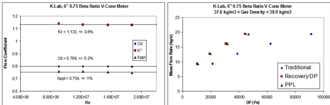
Fig 15. K-Lab Wet Gas Flow Facilities 6", 0.75 Beta Ratio V-Cone Meter Dry Gas Data.
