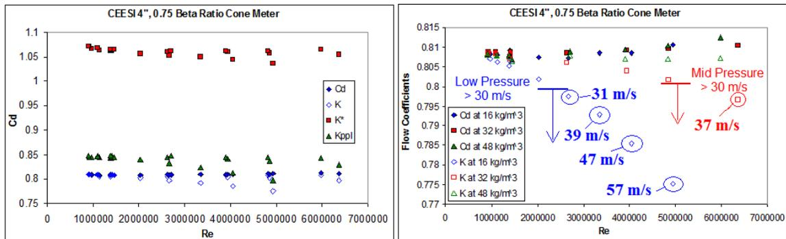
Fig 28. All CEESI Air Blow Down 4", 0.75 Beta Ratio Cone DP Meter Dry Gas Data.
