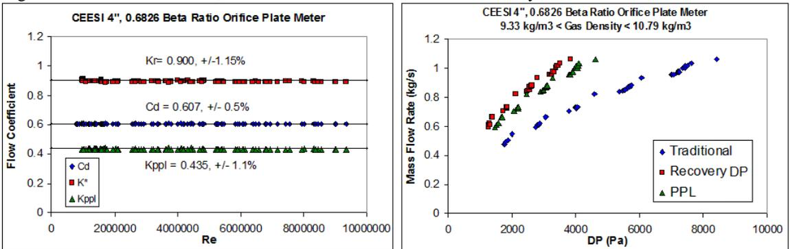
Fig 10. CEESI Wet Gas JIP 4", 0.6826 Beta Ratio Orifice Plate Meter Dry Gas Data.
