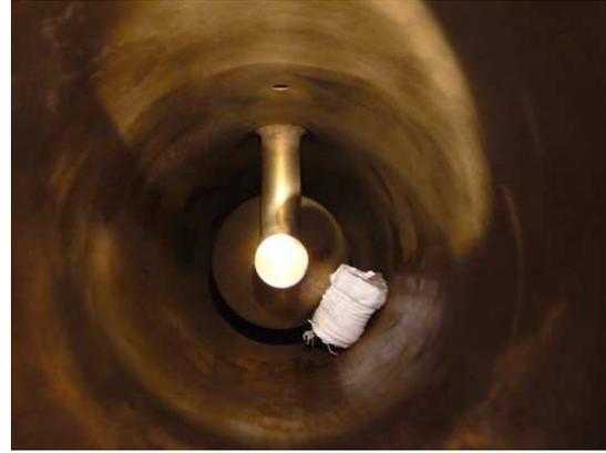
Fig 37b. Cone DP Meter with Partial Blockage
