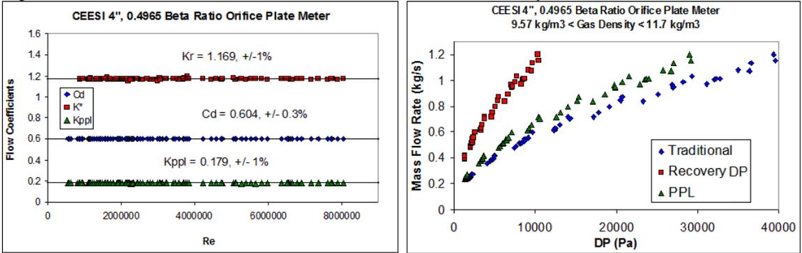
Fig 9. CEESI Wet Gas JIP 4", 0.4965 Beta Ratio Orifice Plate Meter Dry Gas Data.
