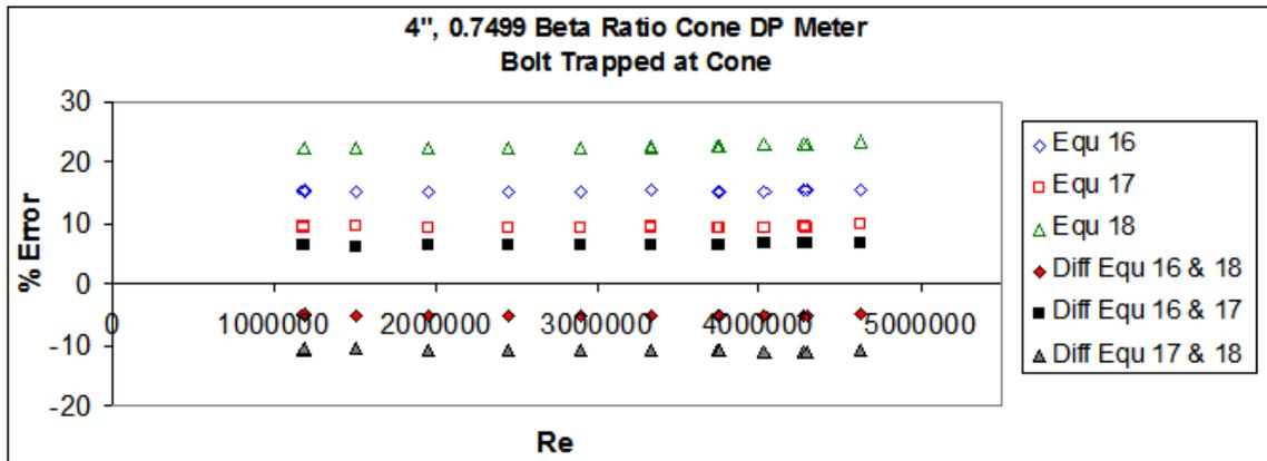
Fig 38. 4", 0.7499 Beta Ratio Cone DP Meter with Bolt Lodged at Cone Element.
