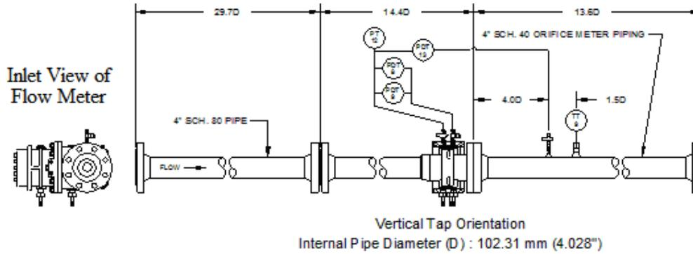
Fig 6. The CEESI JIP orifice meter set up.
