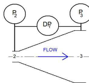
Fig 2. Generalised Expansion DP Meter
