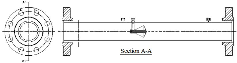
Fig 14. A Sketch of a Generic Cone DP Meter.
