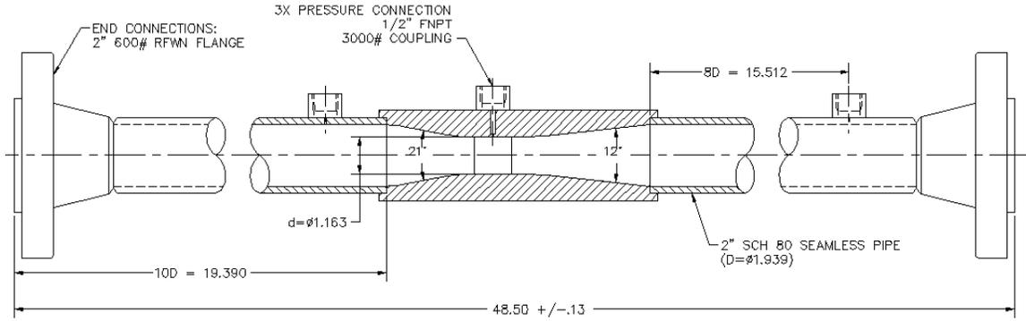
Fig 11. 2", 0.6 Beta Ratio Venturi Meter
