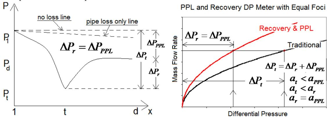
Fig 5c. Pressure fluctuation through DP meter where DP lost and recovered are equal (PLR = 1/2) and the associated three parabolic flow rate equations.
