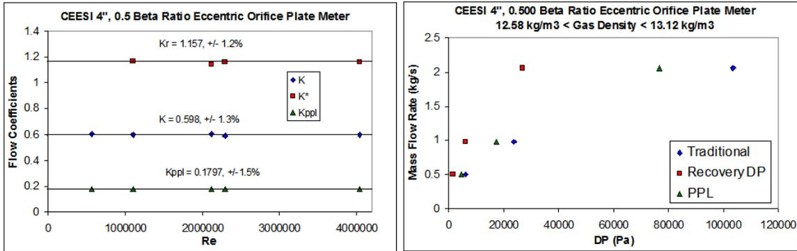
Fig 21. CEESI Wet Gas Facilities 4”, 0.500 Beta Ratio Eccentric Orifice Plate Meter Dry Gas Data.
