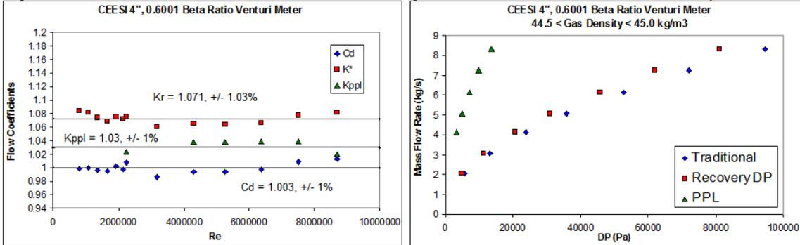
Fig 13. CEESI Wet Gas Flow Facilities Commissioning 4", 0.60 Beta Ratio Venturi Meter Dry Gas Data.
