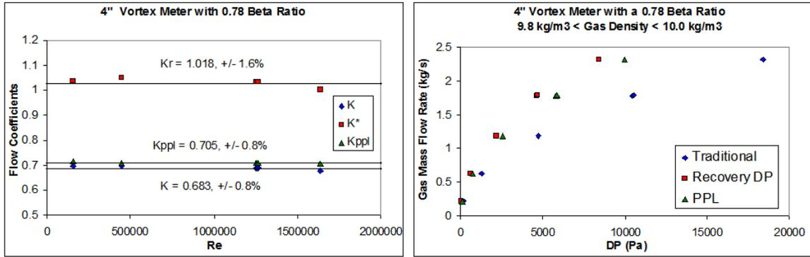
Fig 23. Low and Moderate Velocity CEESI Test Data on Vortex Meter Set Up as a DP Meter.
