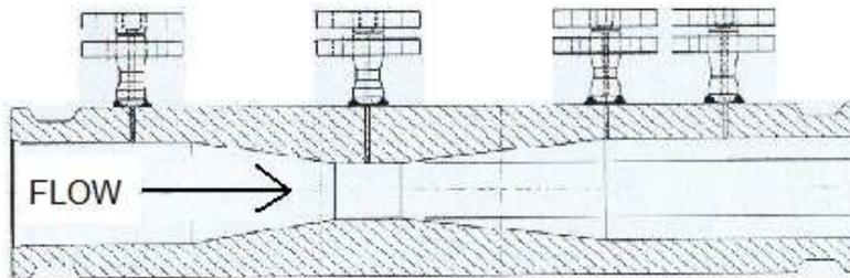
Fig 24. ISA Controls, 6", 0.55 Beta Venturi Meter Tested at NEL.
