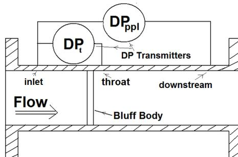
Fig 22. Sketch of the Vortex Meter with Two DP Transmitters Installed.
