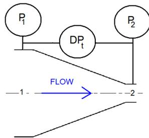
Fig 1. Generalised Constriction DP Meter
