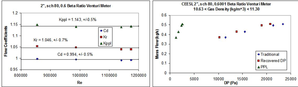
Fig 12. CEESI Wet Gas Flow Facilities Commissioning 2", 0.60 Beta Ratio Venturi Meter Dry Gas Data.
