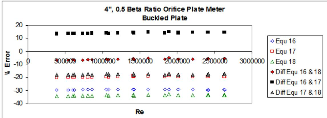
Fig 35. CEESI 4", Sch 40, 0.5 Beta Ratio Orifice Plate Meter with a Buckled Plate.
