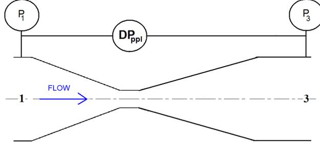
Fig 3. Generalised Permanent Pressure Loss Meter (Venturi sketch not to scale or dimensionally precise.)
