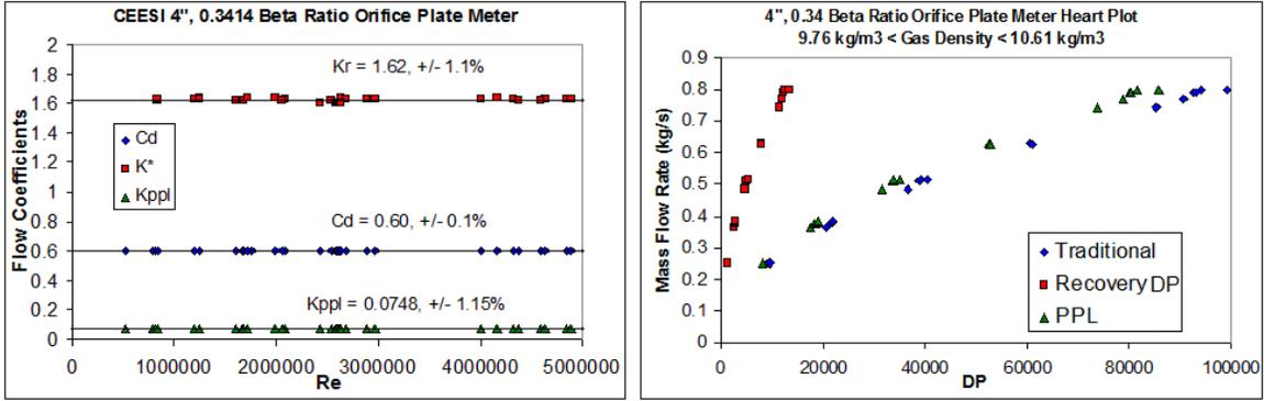
Fig 7. CEESI Wet Gas JIP 4", 0.3414 Beta Ratio Orifice Plate Meter Dry Gas Data.
