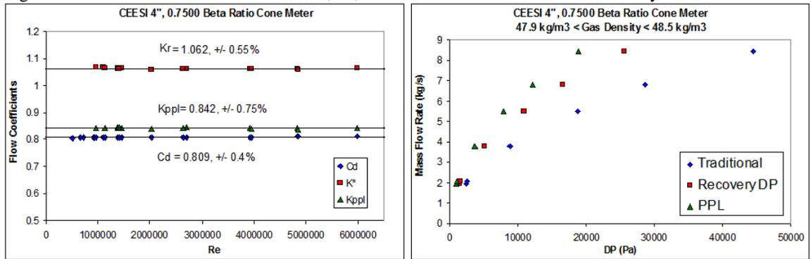
Fig 17. CEESI Air Blow Down 4", 0.7500 Beta Ratio Cone DP Meter Dry Gas Data.
