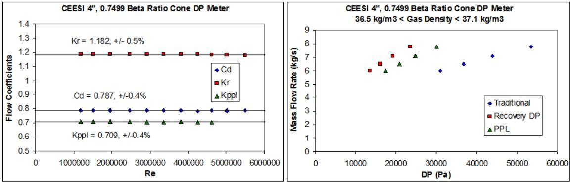
Fig 16. CEESI Air Blow Down Calibration, 4", 0.7499 Beta Ratio Cone DP Meter Dry Gas Data.
