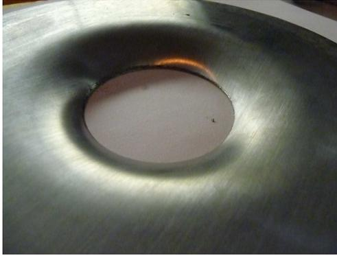
Fig 33a. Buckled Plate (sharp edge upstream)
