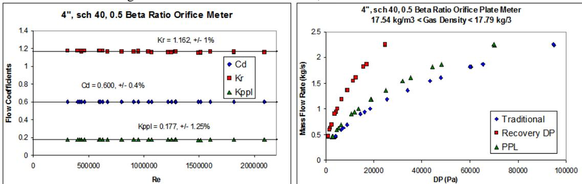
Fig 32. CEESI 4", Sch 40, 0.5 Beta Ratio Orifice Plate Meter Air Blow Down Base Line Test.
