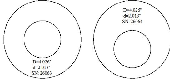
Fig 19. Standard & Eccentric Orifice Plate Designs.
