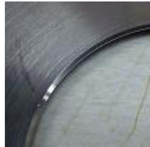
Fig 20. Chamfered (0.02”) orifice edge.
