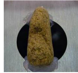
Fig 30. Rock trapped at an orifice plate.
