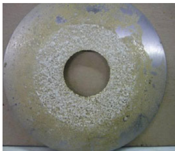
Fig 23. A heavily contaminated orifice plate.
