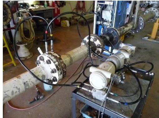
Fig 5. Flange installed plate with air flow.
