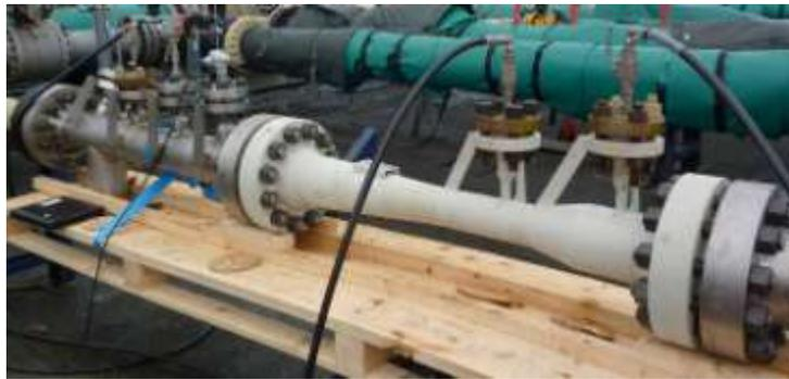
Fig 17. 6", 0.4 Beta Ratio Venturi meter (S/N 2009080-1) at GL Flow Centre.
