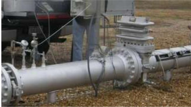
Fig 51. 12”, 0.476  $\beta$  orifice meter prior to Prognosis system installation.
