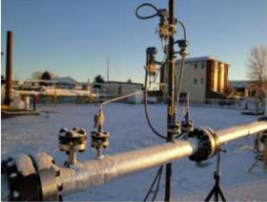
Fig 33. Venturi meter under wet gas tests, CEESI.
