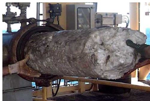
Fig 8b. Hydrate plug in a production line.
