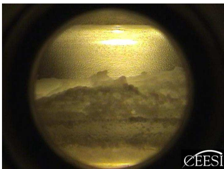
Fig 8a. Wet gas flow hydrate formation.
