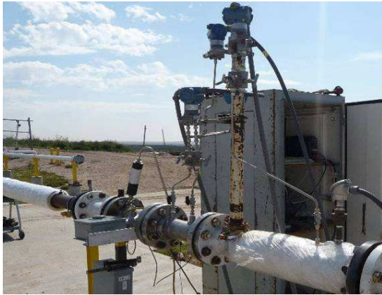
Fig 4. Venturi meter in the CEESI wet gas facility.
